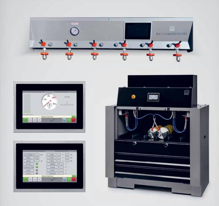
Filling ramp with 6 direct or hose connections for a pressure range 200 or 300 bar. The filling ramp can be integrated to any commercially available breathing air filling system. The filling connections consist of self-venting toggle valves. Filling pressure indication by means of a class 1.6 0-400 bar stainless steel high pressure gauge filled with glycerine.
