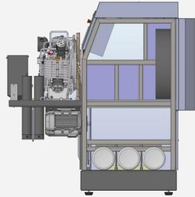
A safety filling box integrated into the line with three filling stations protects against bottle bursting during the filling process. When the con-
